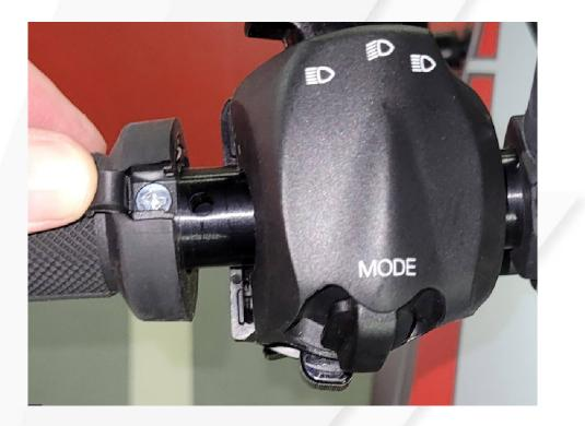
9. Slide on the Cruise Control button. Keep the protruding part of the buttons to the left, see below.
